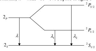
$$E = \frac{hc}{\lambda} \Rightarrow \Delta E = -\frac{hc}{\lambda^{2}} \Delta \lambda = -\frac{1.24 \times 10^{-6} (ev - m)}{(6521 \times 10^{-10} m)^{2}} \times 0.14 \times 10^{-10} m$$
